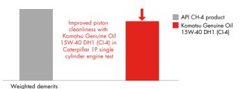
Weighted demerits = overall rating of piston cleanliness, i.e., carbon and lacquer deposits – a lower number is better
