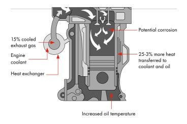
EGR increases heat transfer and potential corrosion, so the lubricant must prevent corrosion and oil oxidation
